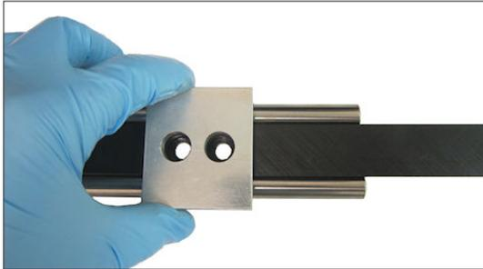
**Step #6** Press cap firmly over rods to bring the "V" groove of each rail into alignment.
