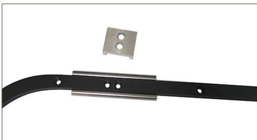
**Step #4** Align aluminum cap with rail holes and the 1/2" diameter rods.
