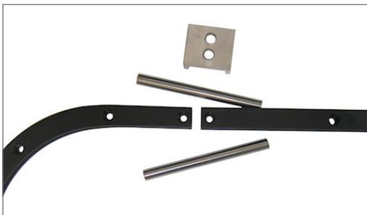
**Step #2** Align rods with "V" groove in each rail as shown.
