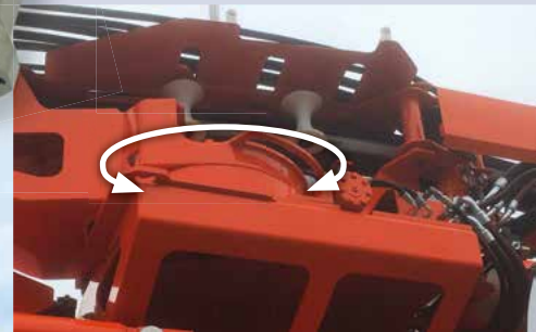
Here, in this high pressure rinsing and suction vehicle , a WD-L 0419 slew drive slews and positions the boom arm for drain cleaning work.
