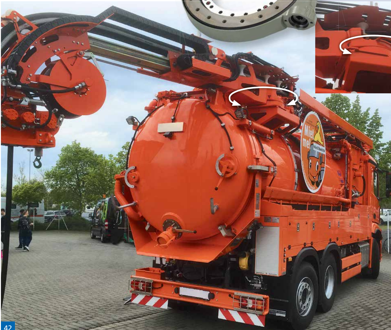
Here, in this high pressure rinsing and suction vehicle , a WD-L 0419 slew drive slews and positions the boom arm for drain cleaning work.
