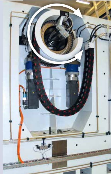
A WD-H 0645 is the central rotation element in this pallet changer for a 5-axis machining center .
