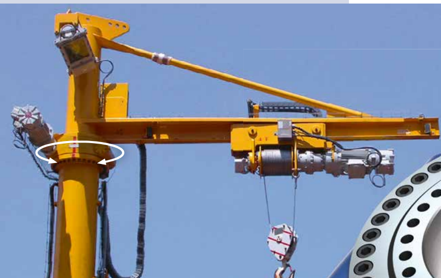
This crane is rotated by a slew drive of the WD-H 0373 series.
