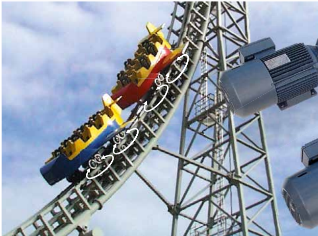
The gondolas of the roller coaster are rotated using a WD-HE 0373 slew drive.
